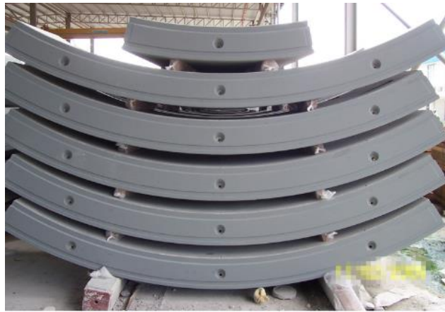
Figure 6.4 Loading condition during the stacking phase (ACI 544.7R, 2016)
